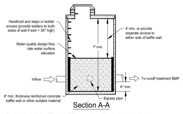
Note: The outlet pipe to the Runoff Treatment BMP may require an orifice plate installed on the outlet to control the water quality design flow rate water surface elevation (weir height). The water quality design flow rate water surface elevation should be set to provide a minimum headwater/diameter ratio of 2.0 on the outlet pipe.
