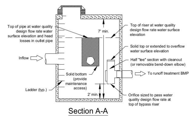
\*Note: Diameter of standpipe (2d) should be large enough to minimize head above water quality design water surface and to keep water quality design flows from increasing more than 10% during 100-year flows.
